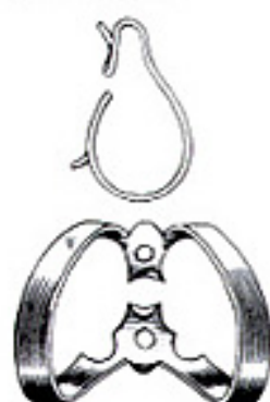
666-36 fig-211 Universal clamp for labial cavities on anterior teeth and bicuspid.
