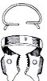
666-06 fig-12A Right and Left Molars. Particularly well-suited for third molars, but also useful for all lower molars. Serrated jaws. Offset jaw height provides stability over a wide range of conditions, including partially-erupted teeth.
